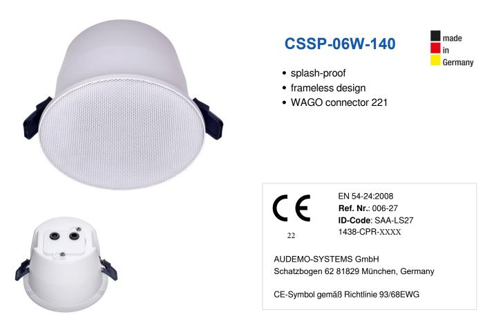
The CSSP-06W-140 is a splash-proof version of the SE-Series which is perfect for the installation in bathrooms, pool areas, e.g. The 6W powered speaker is equipped with a 100mm full-range loudspeaker and a 100V transformer with 3 power adjustments. The powder coated metal in RAL 9016 guarantees long-term stability.
